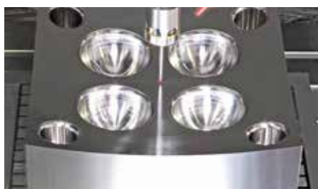
Inspect the Remaining Stock on the Machine
