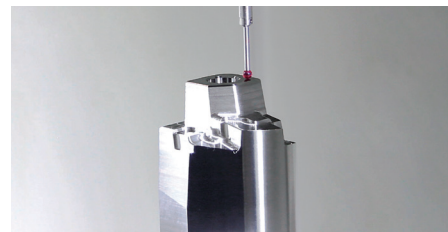
02-Obtain Actual Position on the Machine
