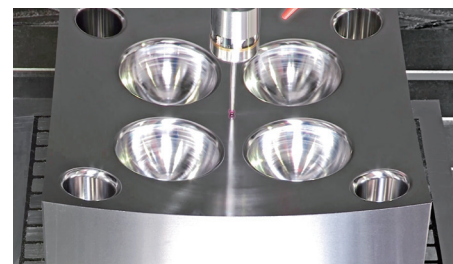
Inspect the Remaining Stock on the Machine
